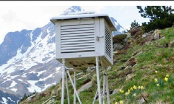
Weather stations are susceptible to variations because of direct weather - like cool breezes or intense direct sunlight. To minimise the effects of these on readings, meteorologists shelter their instruments inside a box called a Stevenson screen.
